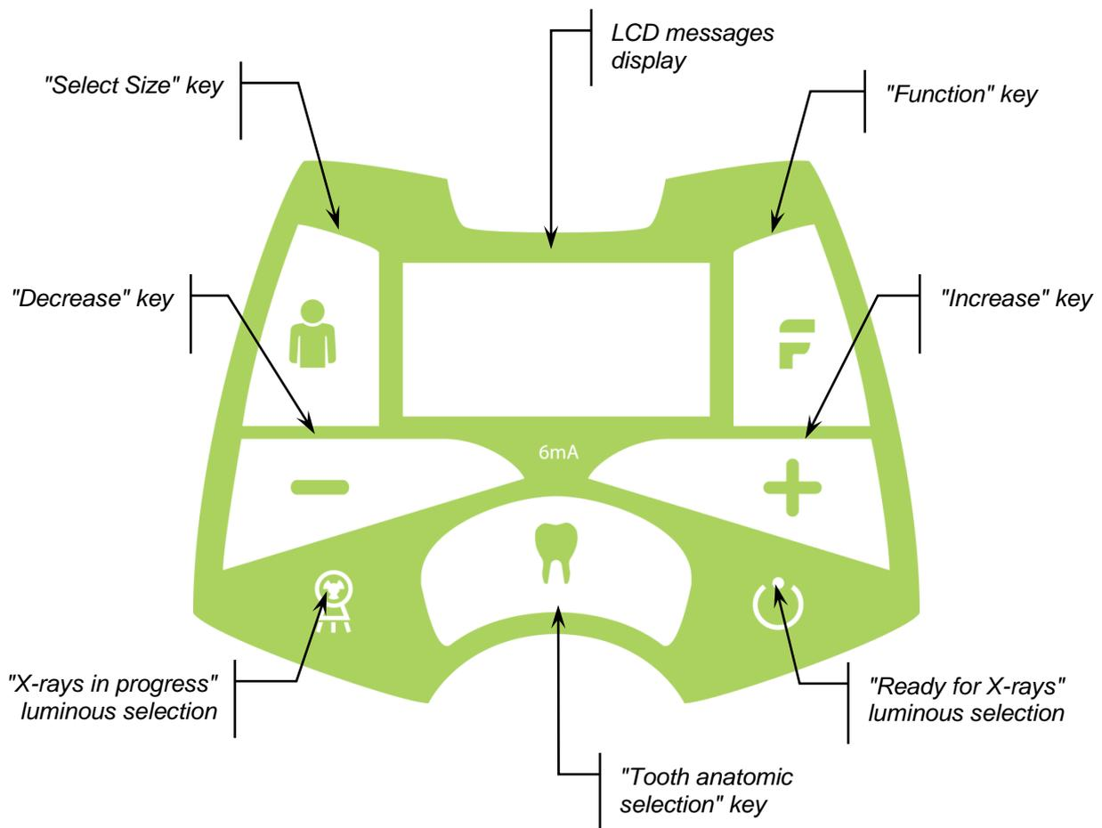
*Figure 8: Duray DC X-Ray Unit control keypad*
