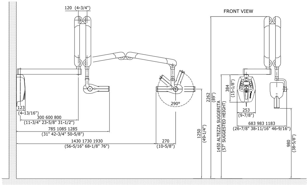
Figure 6: Dimensions of the wall version
