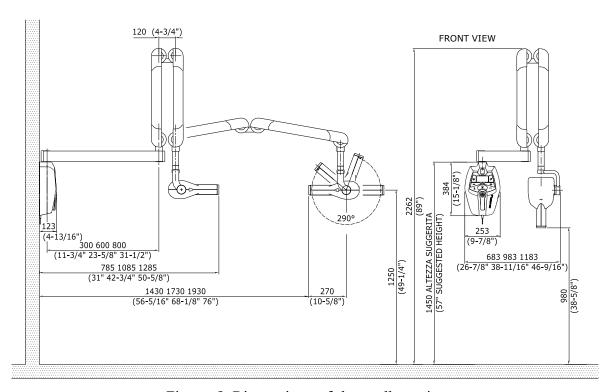
Figure 6: Dimensions of the wall version
