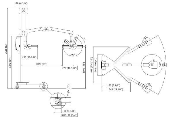
Figure 7: Dimensions of the mobile stand version
