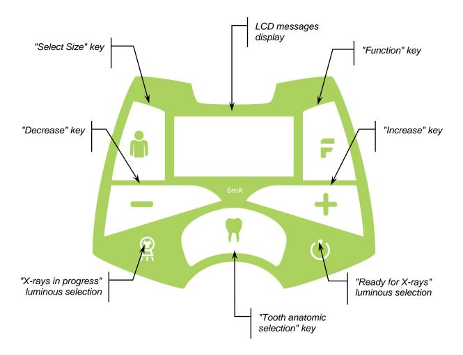
Figure 8: Duray DC X-Ray Unit control keypad
