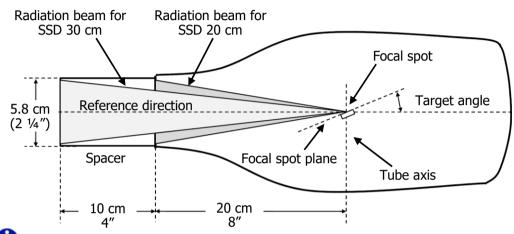
Note. The position of the focal spot is marked on the outside of the tube-head with a dot embossed on the top and bottom covers.
