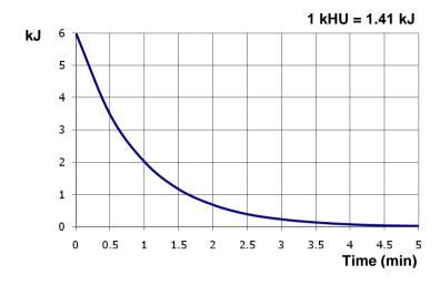
Tube Head Cooling curve
