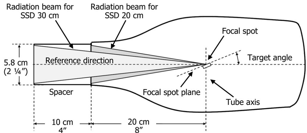
**i** Note. The position of the focal spot is marked on the outside of the tube-head with a dot embossed on the top and bottom covers.
