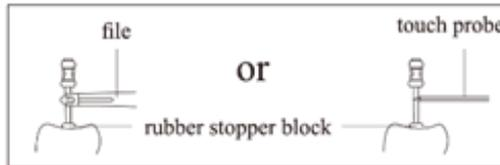
6. Autoclave the lip hook, file clip or touch probe after use
