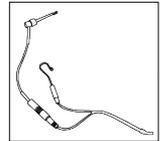
To remove lip hook or file clip, hold the jack and pull apart. Do not pull the wires.
