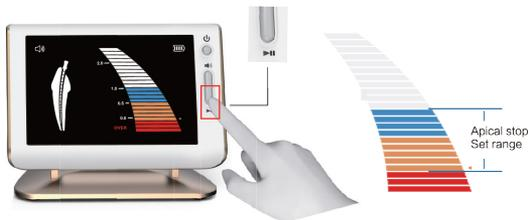
During operation when the file reaches the Apical Stop, the device will beep continually.
