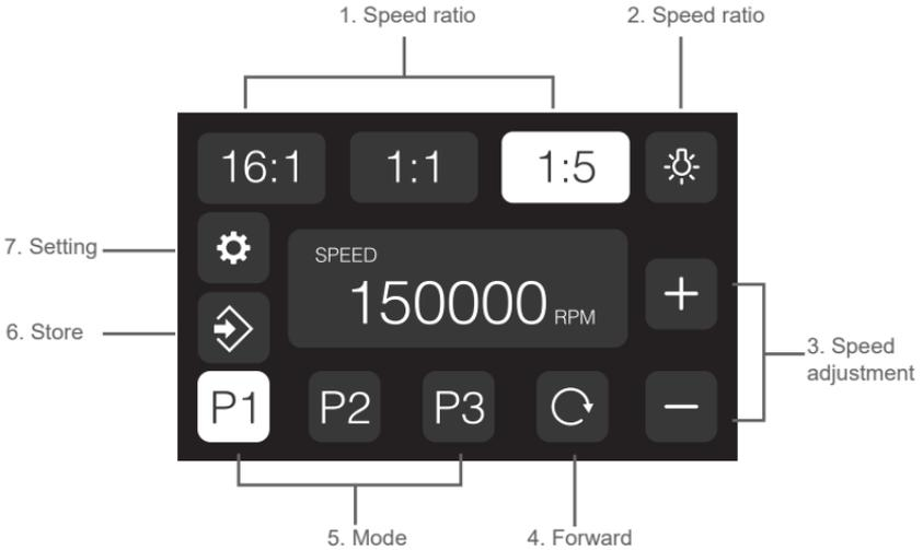
5.6.1 Select speed ratio by through touching key “1”. The color of the key will change when touching the key.
