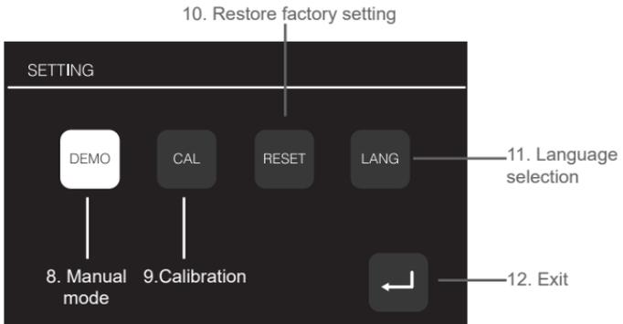
5.7.1 In setting interface, touch key “8” Manual Mode key to enter demo mode interface. Under the demo mode state, the motor rotation can be directly controlled without foot pedal. Touch Speed Ratio key to select corresponding speed ratio. Touch Speed key to adjust the speed. Touch Start key, Stop key, Forward/Reverse Rotation key, and LED key to control the output of motor. Touch the Exit key to exit the demo mode interface.
