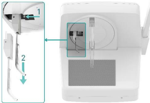
Remove the nasion support by acting on the release pin as illustrated in the side image.
