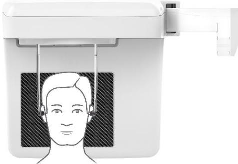
The configuration of the craniostat for Antero-Posterior program is indicated in the side image. Turn the ear plug holder, in order to have ear plug as illustrated in side image. Grasp the holders at the very top with both hands. Push the holders simultaneously outwards as far as they will go. Insert the protective caps for ear plug.
