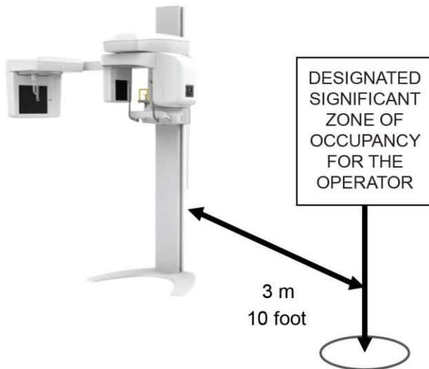
X-ray equipment produces ionizing radiation that may be harmful if not properly controlled. It is therefore recommended that the equipment be operated by trained personnel only, in accordance with existing law.
