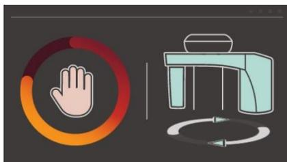
During system initialization the image to the side is shown on the display.
