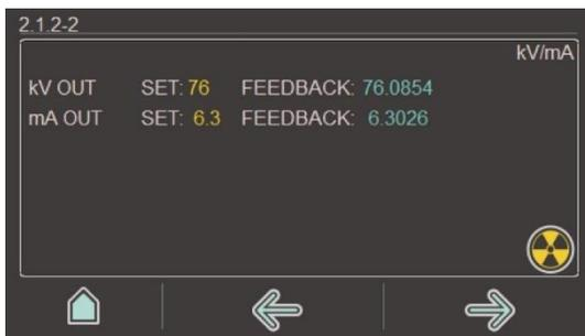
Second page shows status of the feedback signals for kV and mA signal.
