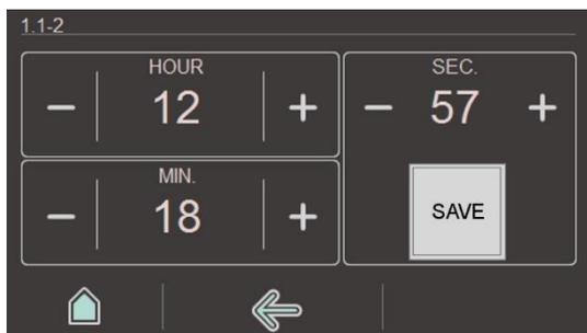
Adjust the time of the device by pressing the “+” and “-” button on the related sections.
