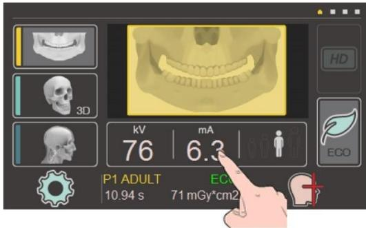
It is possible to select patient size or adjust manually the technical parameters kV and mA (mAs only for cephalometric programs) by pressing the “kV/mA/size” button, in the middle of the display home page.
